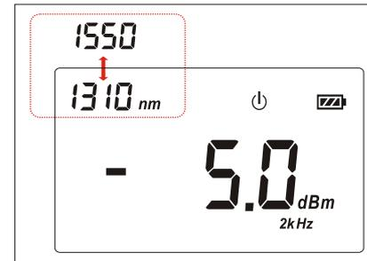
Press the “λ” Key to switch the wavelength between 1310nm and 1550nm.
