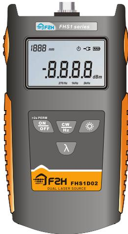
The FHS1D series mini-sized dual-wavelength laser sources offer excellent stability and portability for accurate fiber optic testing. Single output port provides stable laser power at dual-wavelength. The compact unit operates in either continuous wave (CW) mode or modulated mode. A low battery indicator reminds the user of replacing the battery.
